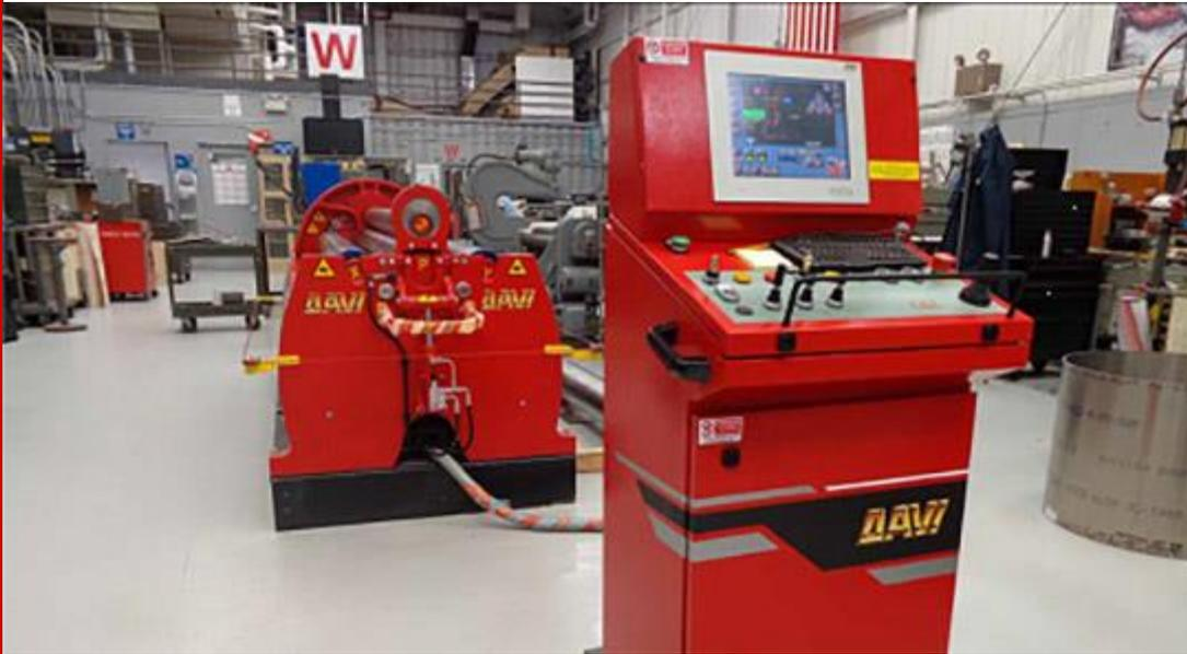
The new 4 roll DAVI inside the JPL-Nasa workshop in Pasadena - California with a successfully rolled part, at the right, on the floor.
